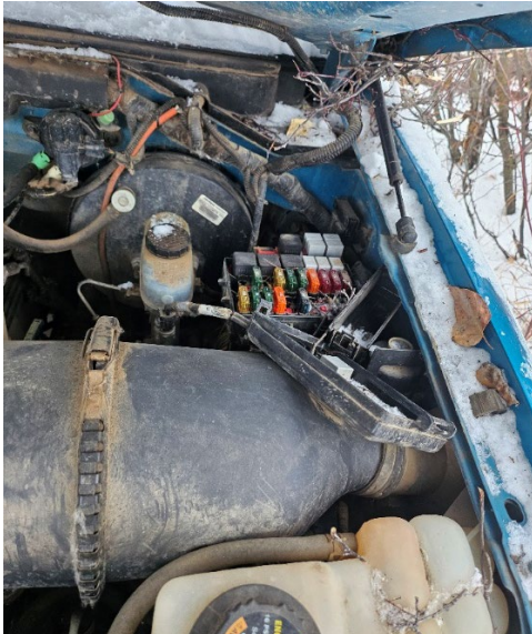
Photo B6 – Engine Compartment Electrical System Damage from Hotwiring
