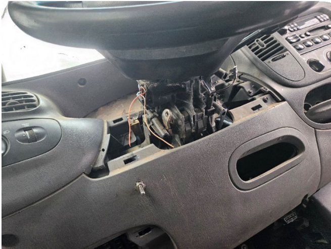
Photo B5 – Additional View of Ignition and Steering Column Damage
